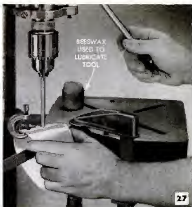
Above, round-end drill rod is chucked in drill press and used to "dimple" rivet hole in light sheet metal. Beeswax is used as lubricant to prevent scoring metal
